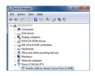
Check that your computer recognizes the adapter in the Device Manger
